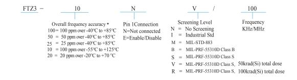
\* Overall Frequency Accuracy includes effects of Operating Temperature, Supply Voltage, Load variations and 10 year aging
