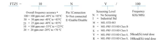
\* Overall Frequency Accuracy includes effects of Operating Temperature, Supply Voltage, Load variations and 10 year aging
