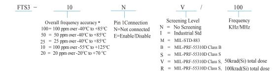
\* Overall Frequency Accuracy includes effects of Operating Temperature, Supply Voltage, Load variations and 10 year aging
