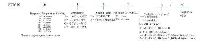
P/N Example: FTTC15 -10DHTV - 50.000 MHz = 50.000 MHz, Class "V" Oscillator, + 1 PPM Overall Frequency Accuracy over an operating temperature range of -40 °C to +85 °C, 3.3V,HCMOS output,TCXO
